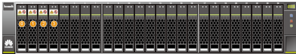
Figure 4-129 Positions of external coffer disks in the disk and controller separation architecture
