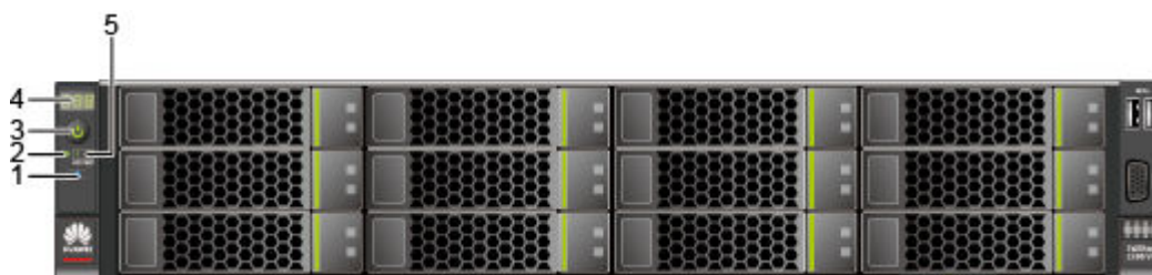
Figure 4-136 Indicators and buttons on the front panel of a server with 12 x 3.5-inch disks
