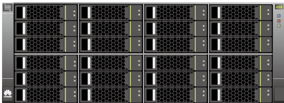
Figure 4-6 4 U disk enclosure with 24 disk slots
